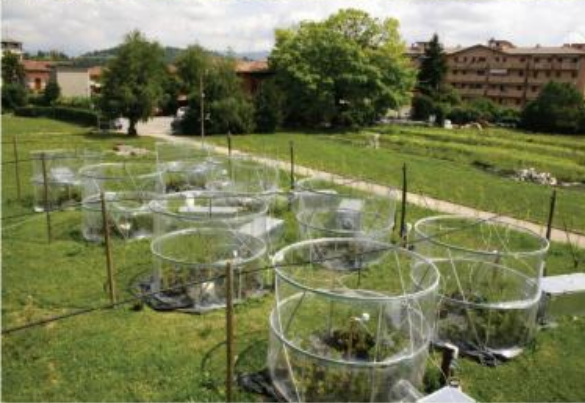
Ozone exposure experiments using open-top chambers in Spain and Italy
